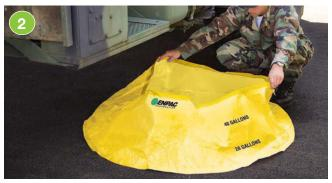
Step 2: Position pool underneath spill source.
