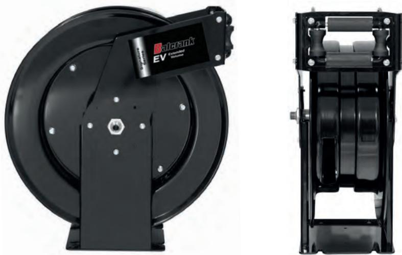
The Extended Volume, EV Series hose reels are designed for high volume heavy-duty applications where large hose diameters are required for increased flow. The EV reels will accommodate up to 50' of 3/4" ID hose or 65' of 1/2" ID hose. Perfect for heavy-duty fleet, construction, mining and industrial applications. All EV series reels include hose, hose stop and a 2.5' connecting hose.
